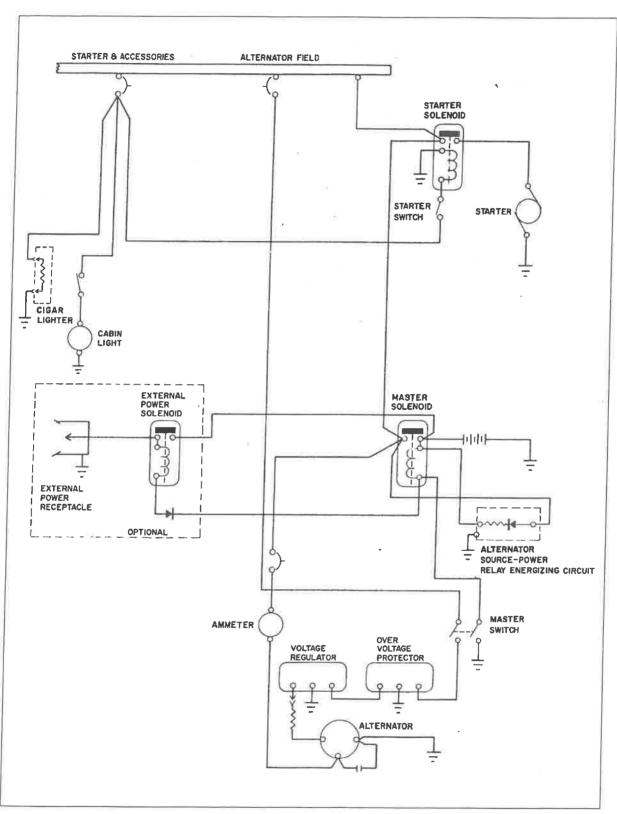
Alternator and Starter Schematic (Ser. nos. 7405001 through 7405290)
